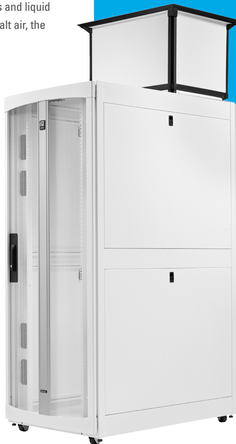
Figure 6: Example of a Type 1 (IP20) enclosure (cabinet) typical of the style used to house compute and data storage equipment in controlled environments such as data centers and computer rooms. Doors are vented to allow front-to-rear airflow. In some instances, ducting is used to guide hot air away through the top of the cabinet. Photo of CPI F-Series TeraFrame® Gen3 Cabinet with patented Vertical Exhaust Duct.
