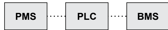
A PLC providing the gateway connection between a building management system and a DCS-based MM PMS is a good example of a combination of controller types
