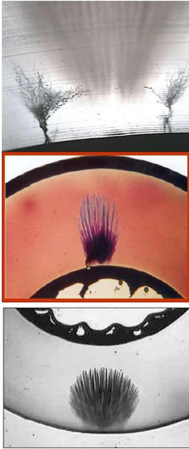
Figure 4. Examples of water trees in power cable insulation
