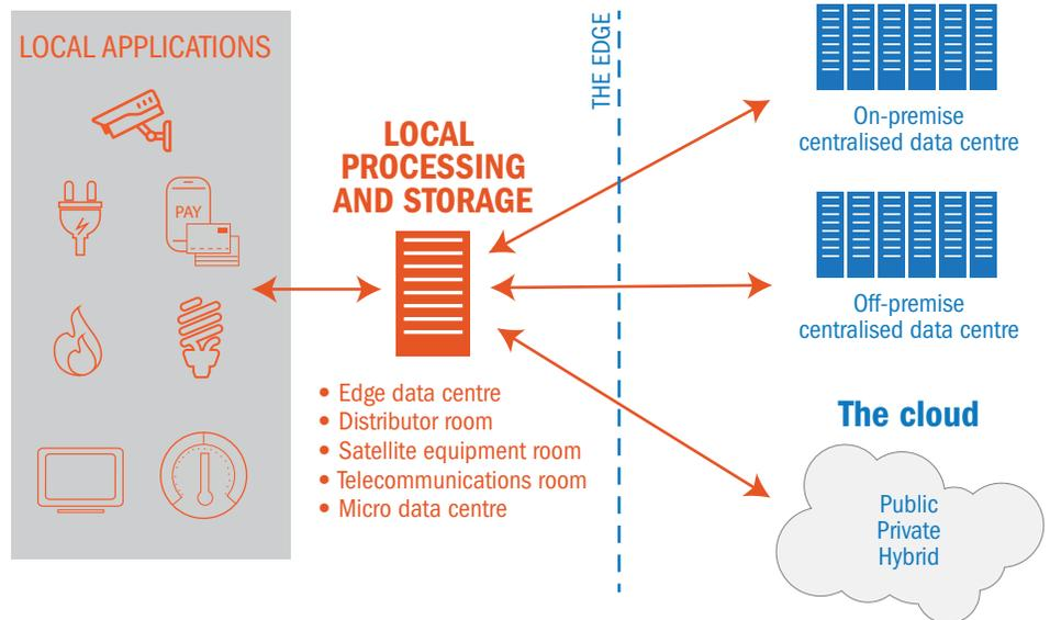
**Edge computing** describes a data centre topology in which information processing and content collection and delivery are placed closer to the sources of this information. The goals are to reduce latency, reduce unnecessary traffic and establish a hub for interconnection between interested peers and for data thinning of complex media types or computational loads.<sup>4</sup>
